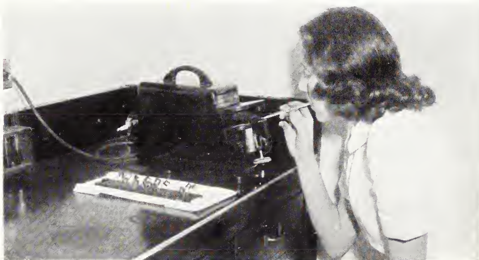
An important instrument in the laboratory is the photoelectric hemoglobinometer, which measures the number of grams of hemoglobin per hundred cc. of blood.
